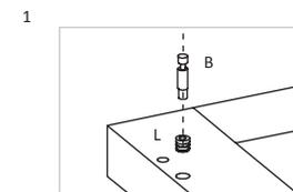
FIXAR BUCHAS DE NYLON NO TAMPO COM AUXÍLIO DO MARTELO DE BORRACHA E PARAFUSAR MINIFIX NA BUCHA
